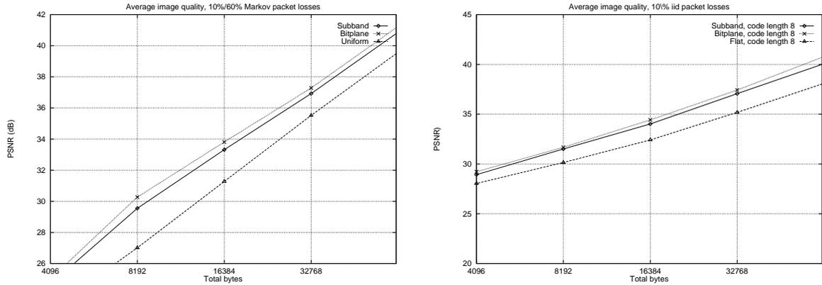
Figure 2: Image quality as a function of the total byte budget. For the plot on the left, packets are erased in bursts following a Markov model: the probability of an erasure is 60% if the previous packet was erased and 10% if not. The benefits of joint source/channel coding are even more pronounced for such a channel than for figure 1. The channel on the right is as in figure 1, but all channel codes are limited to length 8. Again the benefits of joint source/channel coding are enhanced.
