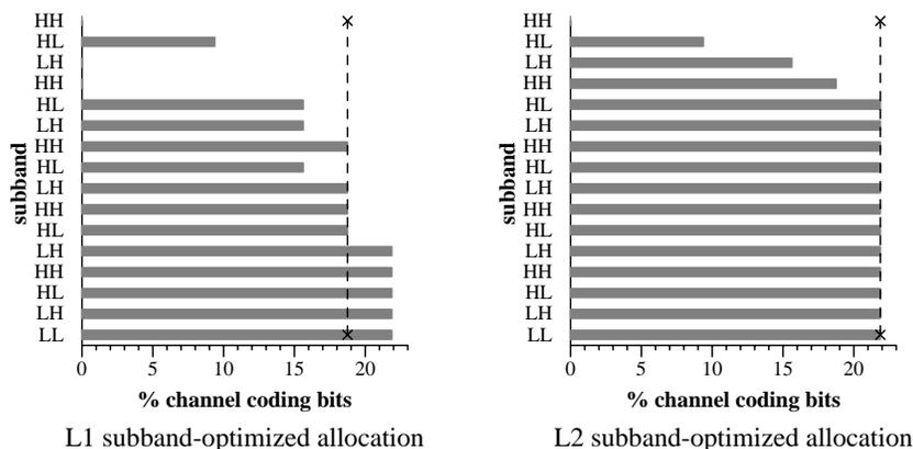
Figure 5: Channel code allocations for  $L^1$  and  $L^2$  optimization. Subbands are from a 5-stage wavelet decomposition and are ordered from coarsest (bottom) to finest (top). The vertical dashed lines indicate optimal uniform channel code levels.
