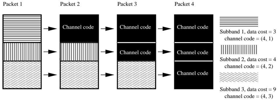
Figure 3: Distribution of data and channel codes into  $N$  network packets. A series of  $(N, k)$  block codes are formed from byte  $j$  of each packet. By varying  $k$  for each byte we can create packets in which data has varying levels of protection.
