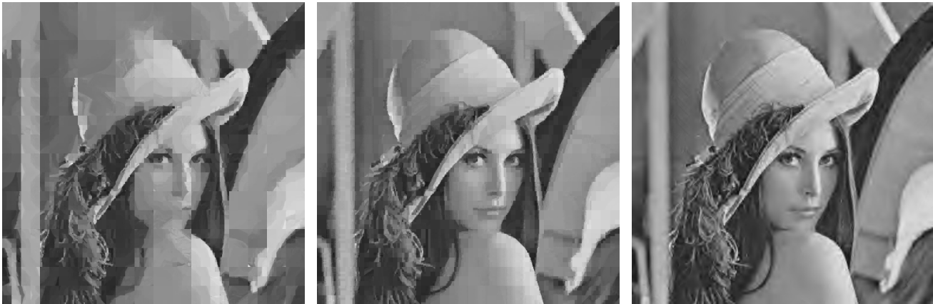
Fig. 5. The leftmost 512 \times 512 Lena image has been compressed at 60.6:1 (PSNR = 24.9 dB) using a disjoint domain pool and the quadtree coder from [18]. The center image has been compressed at 68.2:1 (PSNR = 28.0 dB) using our self-quantization of subtrees (SQS) scheme with the Haar basis. Our SQS scheme uses exactly the same domain pool as the quadtree scheme, but our analysis of the SQS scheme enables us to make much more efficient use of bits. The rightmost image has been compressed at 65.6:1 (PSNR = 29.9 dB) using a smooth wavelet basis. Blocking artifacts have been completely eliminated.
